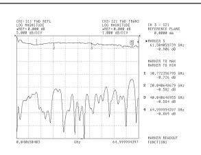
**Figure 4.** Typical V251 Insertion Loss and Return Loss, 40 MHz to 65 GHz
