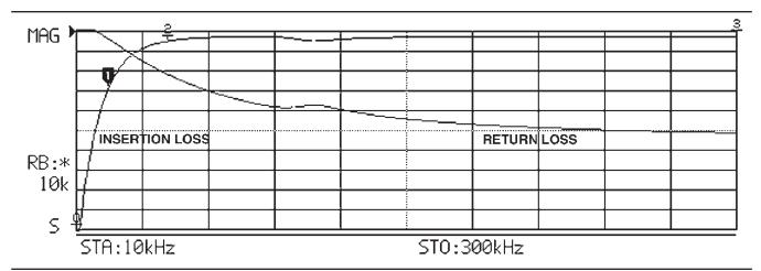
Figure 2. Typical V255 Insertion Loss and Return Loss, 1 kHz to 1 MHz
