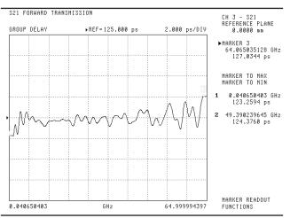
**Figure 6.** Typical Group Delay Performance measured on V255
