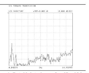
$\label{eq:Figure 3.} \textbf{Figure 3.} \ \ \textbf{Typical Isolation between Data I/P and DC} \\ \textbf{Port}$
